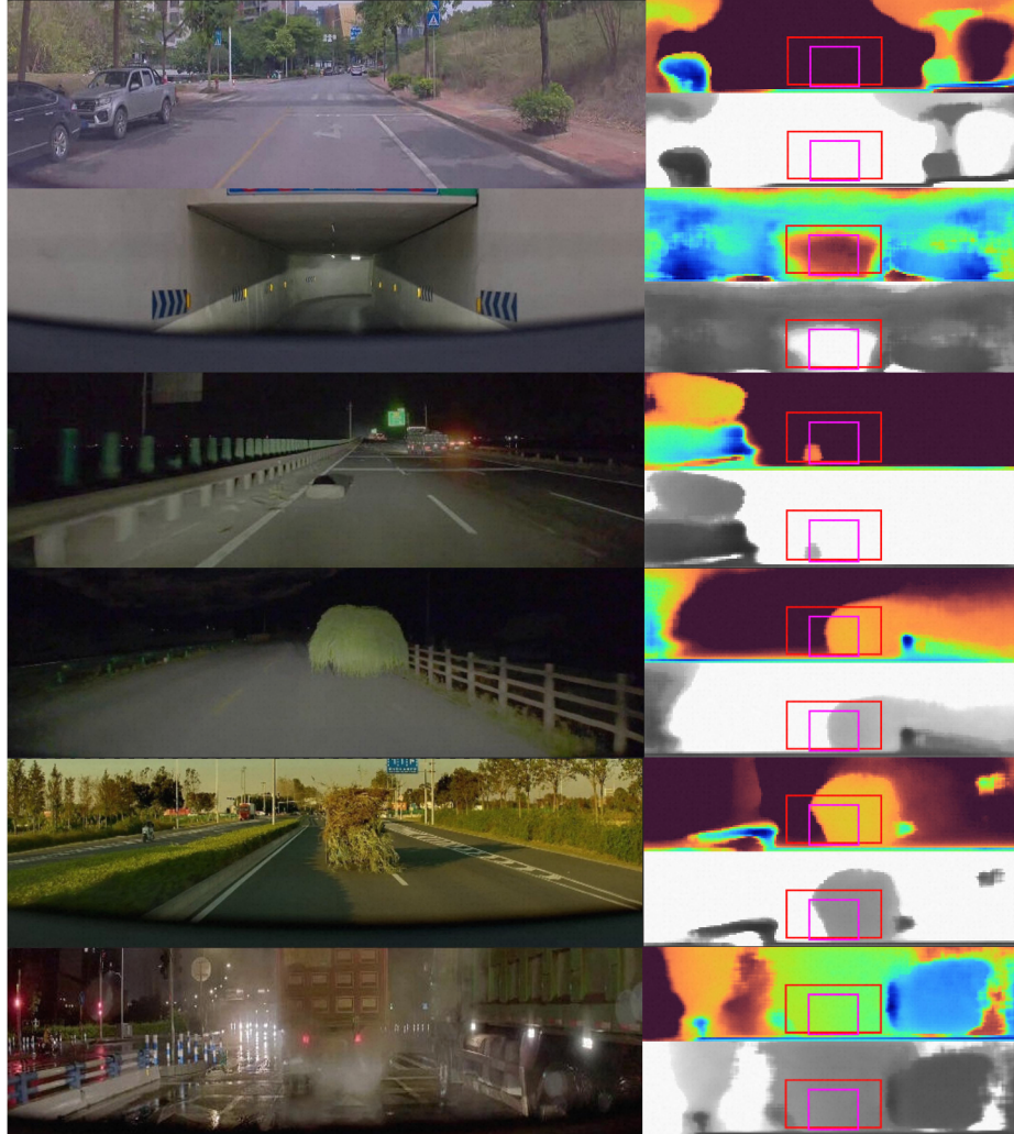
Fig. 3: Qualitative results on real driving scenes. The left column shows the input RGB images. For each example, the right column visualizes the predicted front-view depth map: the top image is a colorized depth rendering, and the bottom image is a grayscale visualization. The red rectangle indicates the evaluation region of interest (ROI), covering a 4m width and a height range of 0.4–2.4m in the ego frame. The magenta rectangle denotes the ego-vehicle body footprint.
